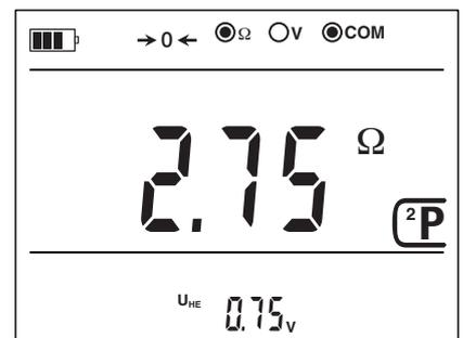
The  $\rightarrow 0 \leftarrow$  symbol blinks during the compensation. When it is done, the display unit indicates **00.00Ω**.
