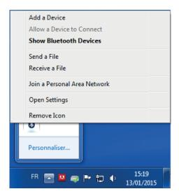
The PC searches its environment for Bluetooth-compatible devices. When the megohmmeter is detected, select it and click Next.
