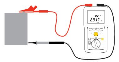
The instrument displays the voltage on the terminals. It detects whether the voltage is AC or DC and, if it is AC, the C.A 6532 also displays the frequency.
