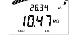
Then long-press the **MEM** key to store the measurement. The measurement is recorded in the first memory slot
