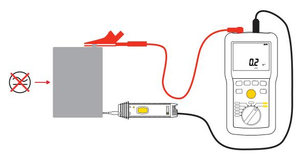
When the probe is connected, the **ID** symbol is displayed.
