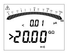
If, during an insulation measurement, the value to be measured exceeds the measurement range (which depends on the instrument and the test voltage), the instrument so reports.
