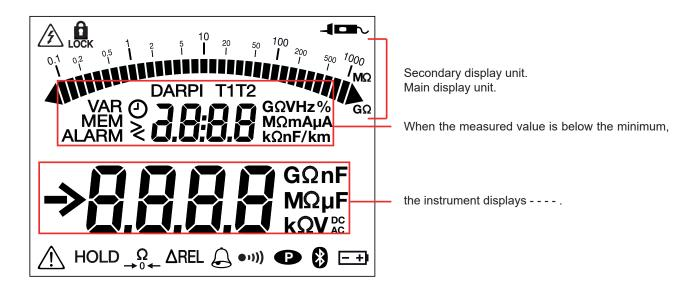
In voltage measurement, when the measurement exceeds the limit (either positive or negative), the instrument displays OL or -OL.
