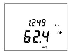
The instrument displays the capacitance and the corresponding line length, computed from the programmed capacitance per unit length.
