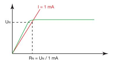
The range of operation per IEC 61557 is from  $100k\Omega$  to  $2~G\Omega$  (see § 4.2).
