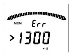
When the memory is full, it is no longer possible to record measurements and the instrument displays the screen shown opposite.
