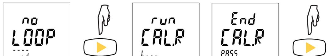
The instrument adjusts the empty clamp. Then it makes the adjustment on an internal resistance of 10Ω. When it has terminated, it displays the result: **PASS** or **FAIL** depending on whether the adjustment succeeded or failed. Press the ► key to terminate.
