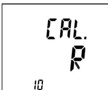
To enter the impedance measurement adjustment procedure, press the ► key for more than 3 seconds. The instrument then alternately displays **NO LOOP** and **PRESS RT** to indicate that the clamp must not be on a conductor. When this condition is met, press the ► key.
