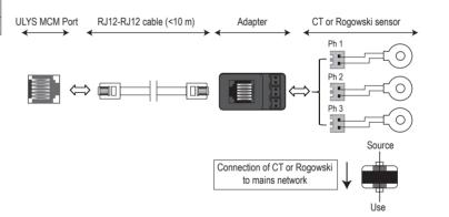
The RJ12 connection cable must be a maximum of 10 m in length and is available from Chauvin Arnoux Energy in several length variants.
