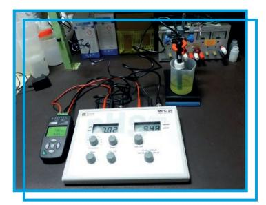
The **L452 Datalogger** can be used with all Chauvin Arnoux electrochemical measuring instruments (analogue and digital)
