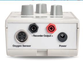
The L452 offers three voltage acquisition modes: 0-100 mV / 0-1 V / 0-10 V. You should use the 0-10 V mode and enter in the instrument the value in % or mg/L at 0 V and the value in % or mg/L for 10 V.
