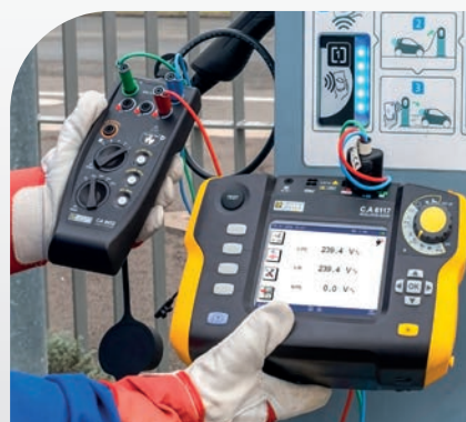
Testing the voltages supplied by a charging station with type-B/ EV 6 mA RCD during charging
