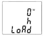
8. To access the screens concerning the energies generated by the load and therefore received by the source ("Supply side"), press the two ;
