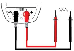
An audible signal is emitted if there is continuity, and the measured value is displayed on the screen.
