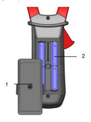
Figure 6: the battery compartment cover
