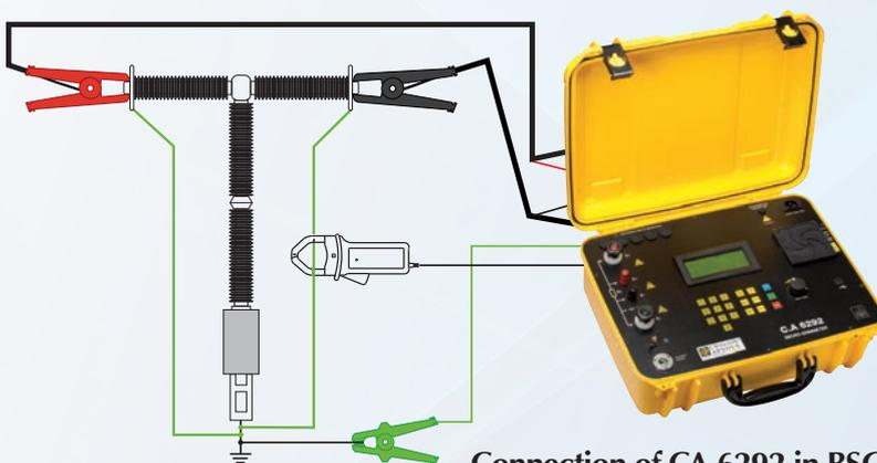
Connection of CA 6292 in BSG measurement mode
