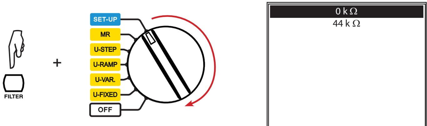
Use the ▲▼ keys to select the compensation and press the ► key to confirm or ◀ to exit.
