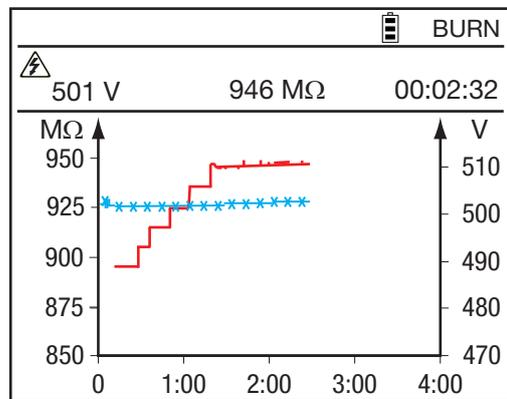
For U-VAR and U-FIXED it is also possible to change measurement parameters during the measurement by pressing the CONFIG key. It is possible to fix the current measurement range, to add an analogue filter, or to change the test voltage if in the variable test voltage mode U-VAR. For more details, refer to § 4.3.
