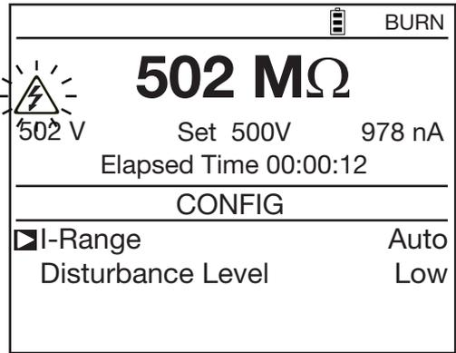
Use the ◀▶ and ▲▼ keys to modify the measurement current range:
