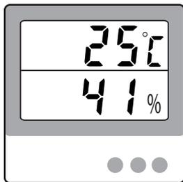
This measurement varies greatly with the temperature and the relative humidity. It is therefore essential to measure them using a separate device (see §1.2) and to record them with the insulation value.
