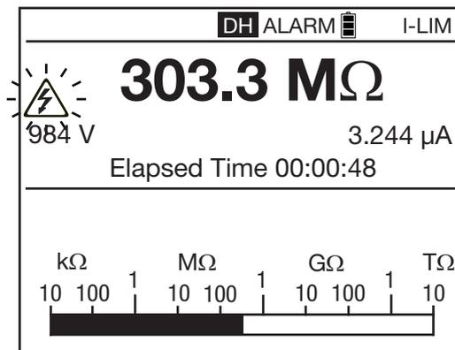
This function is useful in case of high instability of the insulation values displayed, but it is also possible to estimate the measurement on the bargraph.
