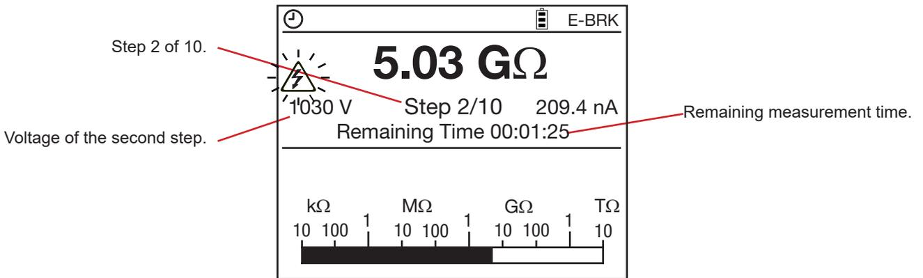
You can view the graphical representation of the measurement results by pressing the GRAPH key. For more details, refer to § 4.5.
