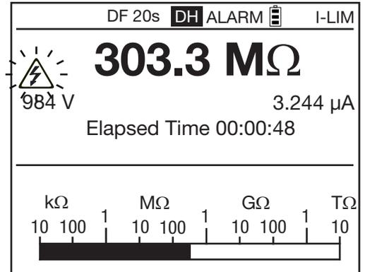
fluctuating high insulation resistance values. Such fluctuations may be due to hand effects, fluctuating capacitances in the device tested, insulation that varies because of conducting dust, an ionizing and polarizing effect of this dust, etc., or again to the presence of an AC voltage superposed on the measurement.
