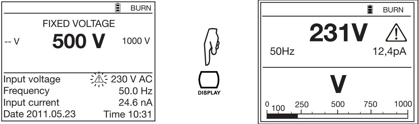
When the external voltage exceeds 25V, the blinking (⚠) symbol is displayed alongside it.
