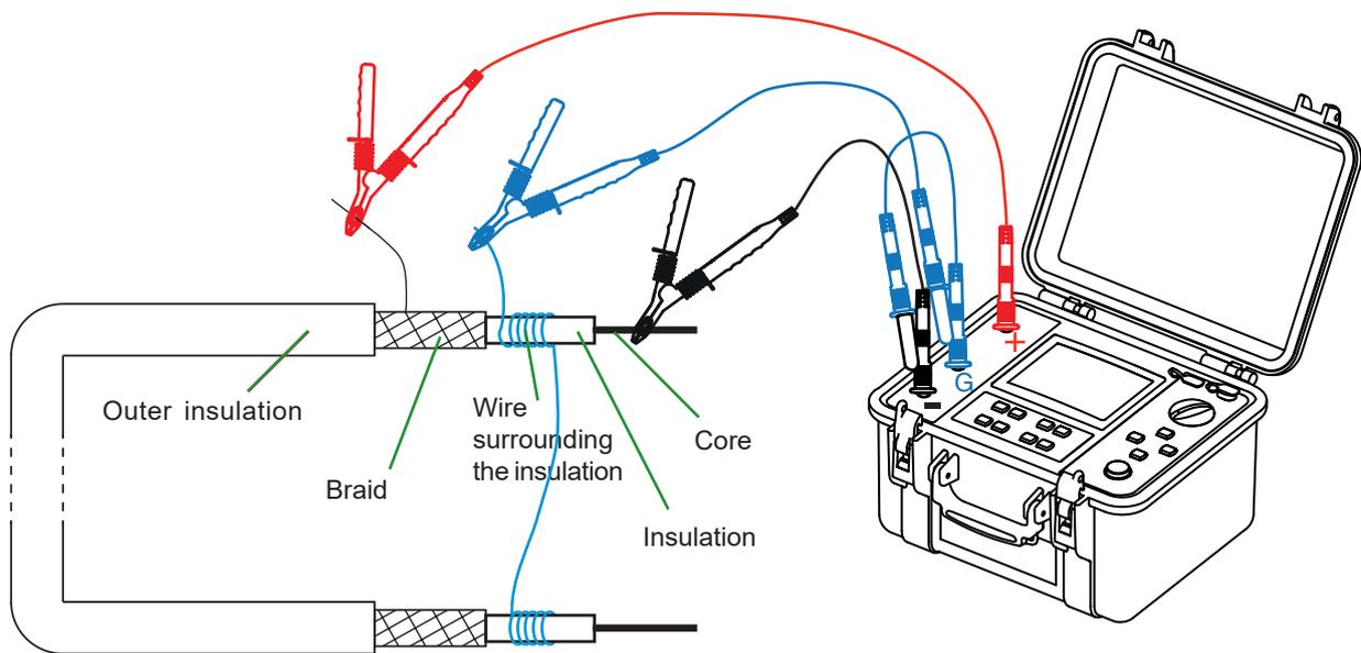
Using the guard eliminates the influence of the surface leakage current.
