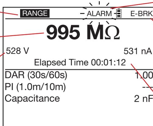
Insulation resistance below the alarm threshold.
