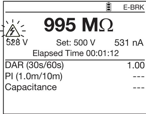
In the case of a step test voltage (10 steps at most) or ramp test voltage (3 steps), the progress of the steps is indicated.
