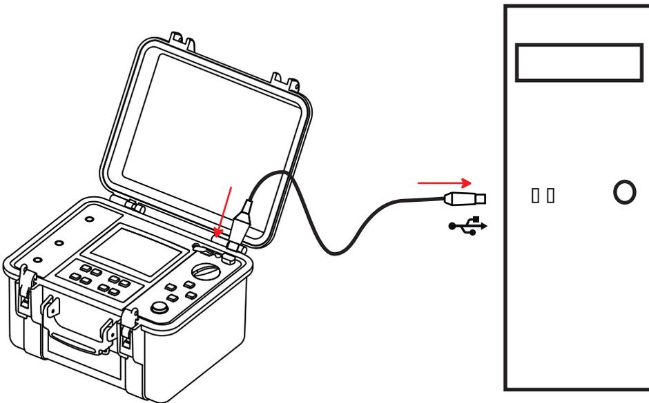
When in communication with a PC, the instrument displays REMOTE and no longer reacts to the user's commands. The keys and the rotary switch are inactive, except for stopping the instrument (OFF setting).
